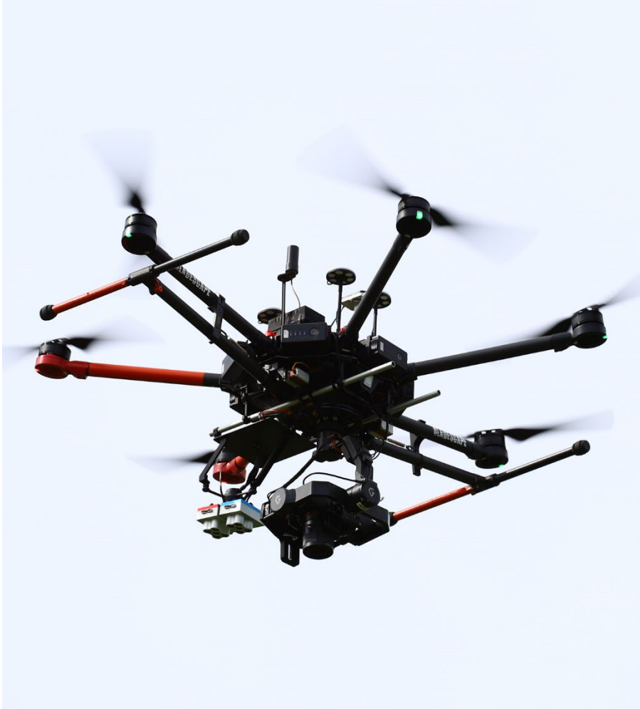
Drone with Sony RGB camera and Micasense multispectral cameras
